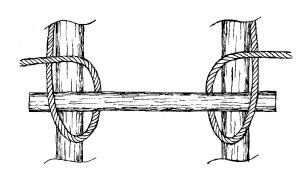
**STEP 3:** Pull the running part side of each overhand loop behind and to the outside of each rail.
