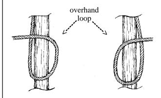
**STEP 2:** Place a rung across the rails so that the standing part of each overhand loop is over the end of the rung and the running part of each overhand loop is under the rung.
