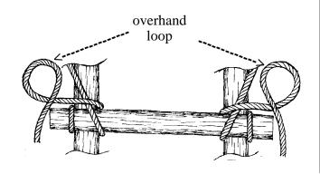
**STEP 7:** Place an overhand loop over each end of the rung to form a half hitch around each end of the rung.
