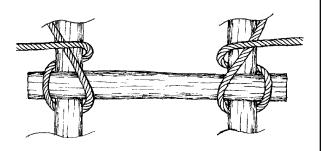
**STEP 5:** Work each rope until it is tightened around the rung and the rung is in its desired position.
